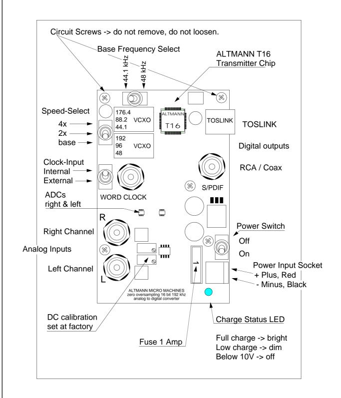
Before charging battery, always disconnect CREATION ADC from battery.
